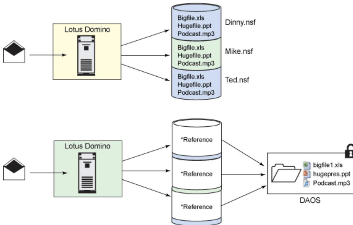
Figure: Previous mail architecture (top panel) and architecture with DAOS (lower panel). Instead of an attachment being stored inside multiple Notes databases, a single attachment is stored as an encrypted file directly in the operating system file structure.
